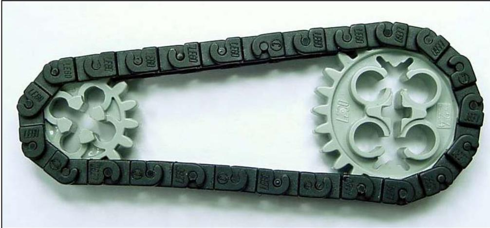
Gear ratios using chain drives are treated just the same as simple machines using meshed gears. Suppose the left gear above has 16 teeth, and the right gear has 24 teeth.
