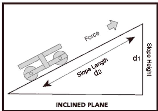
As before, we define *Work* as applying force to move an object a certain distance. An inclined plane reduces the effort necessary to move the load by distributing the force required to perform the task over the distance of the inclined plane. Reducing effort is a good thing, but we do sacrifice having to exert the reduced Force over a greater distance. There's always a trade-off.
