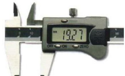
Figure 4 - Digital vernier caliper used to measure inside and outside diameters in either inches or millimeters at a press of a button.
