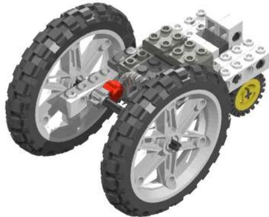
$$\begin{aligned} \omega &= \text{Motor RPM} \times \text{Gear Ratio} \\ &= 300 \text{ rpm} \times 3:1 \\ &= 900 \text{ rpm} \end{aligned}$$
